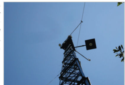
Figure 1. In the detail, top of the Phenology tower showing some devices and the digital fisheye camera (square)
