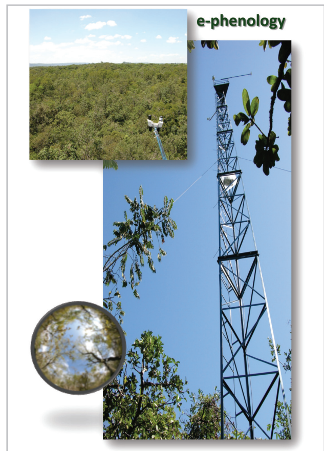
Figure 1. In the detail, top of the Phenology tower showing some devices and the digital fisheye camera (square)
