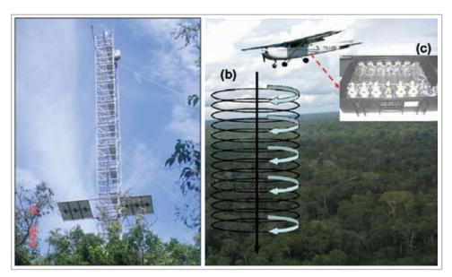
Figure 1. (a) Flux tower over a floodplain area in the ecotonal region of Bananal Island (frontiers of Tocantins-Mato Grosso-Pará); (b) Measurement of atmospheric greenhouse gases with aircraft 's downward sampling using (c) a portable compressor and flask unities
