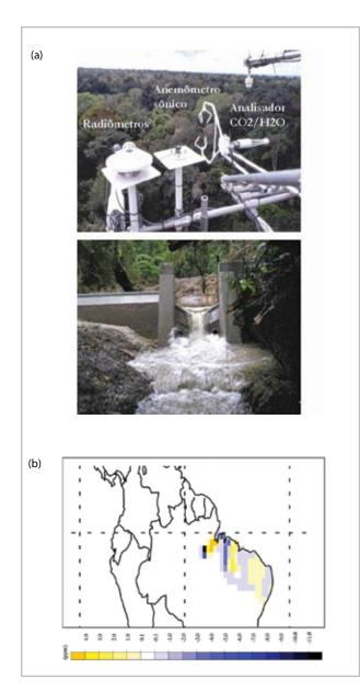
Figure 2. (a) Micrometeorological instrumentation to measure climate, CO<sub>2</sub> flux and evapotranspiration at the top tower, and measurement of basin discharge in the Atlantic Forest; (b) Modelled contribution (in ppm) to the global CO<sub>2</sub> concentration of the surface upwind Santarem, PA
