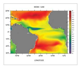
Figure 2: The modeling of river discharges on the global oceans integrates continental hydrology with ocean circulation and biogeochemistry, which in turn impact atmospheric circulation and  $CO_2$  cycles. This figure shows the effect of the Amazon River discharge on equatorial Atlantic sea surface salinity, as simulated by the coupled ocean-atmosphere version of the MBSCG
