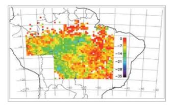
Figure 2. Aerosol radiative forcing at the surface resulting from biomass burning in large areas of Amazonia. A large radiation deficit at the surface of up to -28 watts/m<sup>2</sup> were observed over large areas in Amazonas, with important effects on the ecosystem functioning
