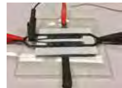
Device detects parts of viral RNA in saliva of infected individuals (photo: UFSCar)
