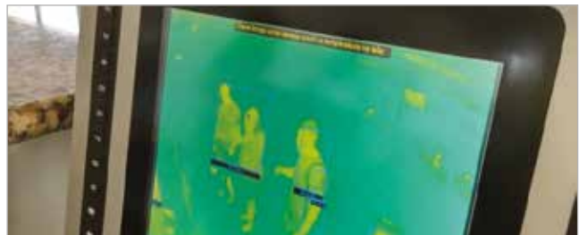
Smart visible and thermal spectrum imaging system to spot people with fever in schools, malls or offices (photo: Opto Space & Defense)
